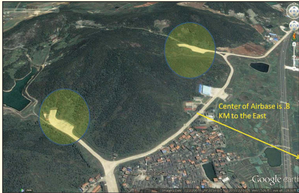
Above: This picture represents the PLA-Navy Yiwu Air Base in Nanjing Military Region. Note the highlighted curved entrances that seek to make it more difficult for a precision guided weapon to make a direct hit.
